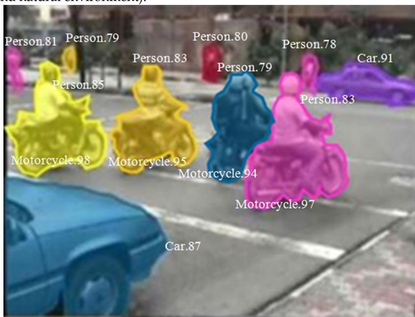
Figure 6: Sample of testing images showing segmentation of cars, motorcycles, persons as road users
