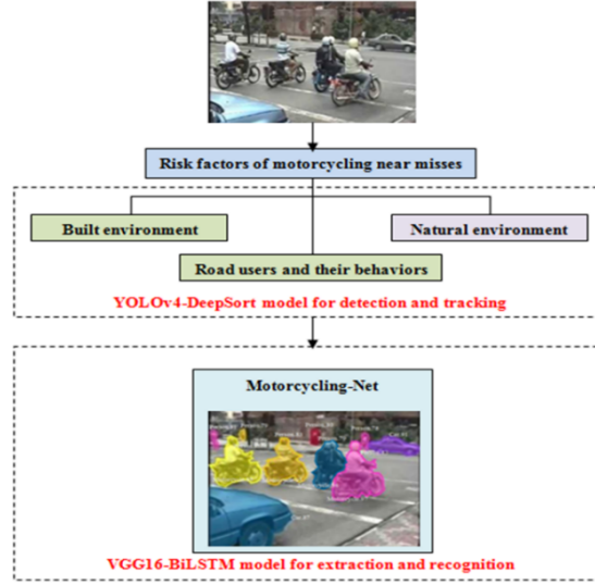
Figure 2: Conceptual framework for understanding near miss's occurrence and detection urban environment
